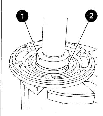
Removing needle bearing in drive end shield (starters with reduction gear only)
